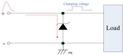
TVS is applied widely in semiconductor and sensitive component's protection. It is usually used in secondary power supply& signal circuit's protection and electrostatic discharge protection in order to prevent IC from over voltage damage.
