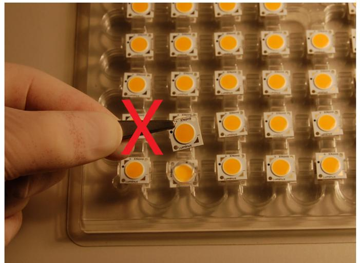
**Fig.5 Incorrect Handling**
