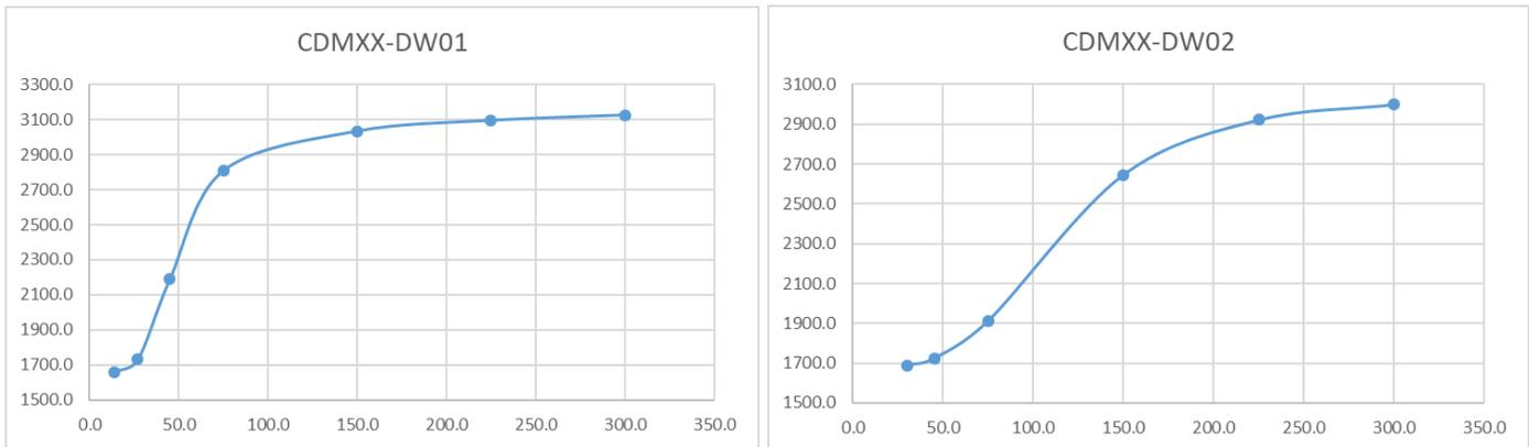
Figure 2: Dimming Curves for Warm Dimming COBs
