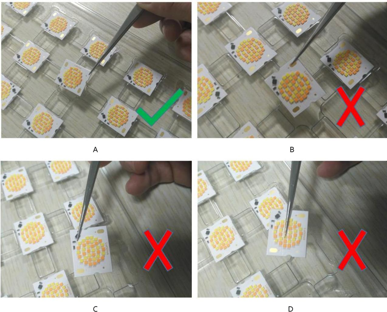
Figure 4: Correct and Incorrect Handling of Dynamic COBs
