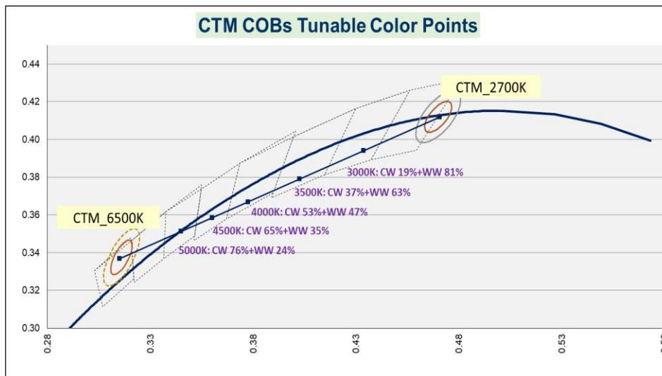
Figure 10B. CW/WW channel current ratio of CTM<sub>6527</sub> at different tunable CCTs
