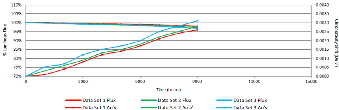
When a luminaire designer uses the MP1616 LM-80 test report to estimate the lumen maintenance of Dynamic COB modules, they should measure the  $T_c$  point of Dynamic COBs in their typical field application conditions then decide which test is the best match to those conditions.
