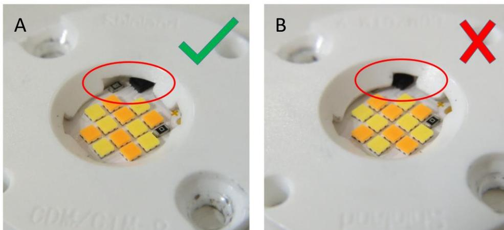
Figure 6: Connector Orientation
