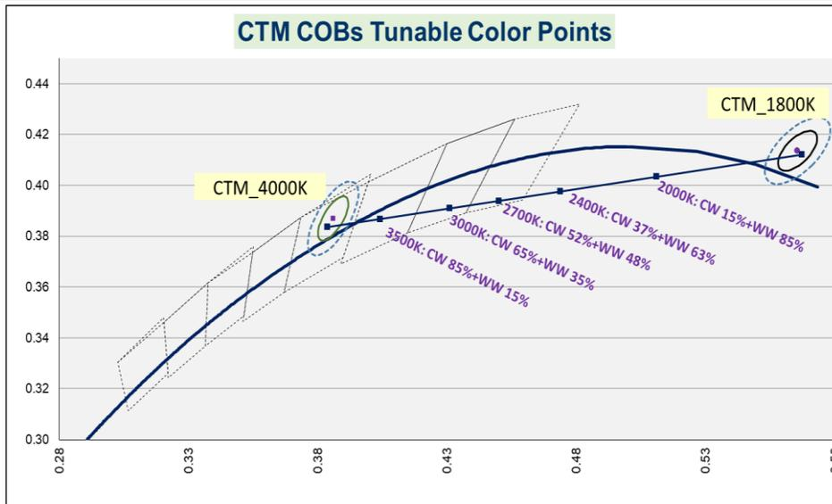
Figure 10A. CW/WW channel current ratio of CTM<sub>4018</sub> at different tunable CCTs
