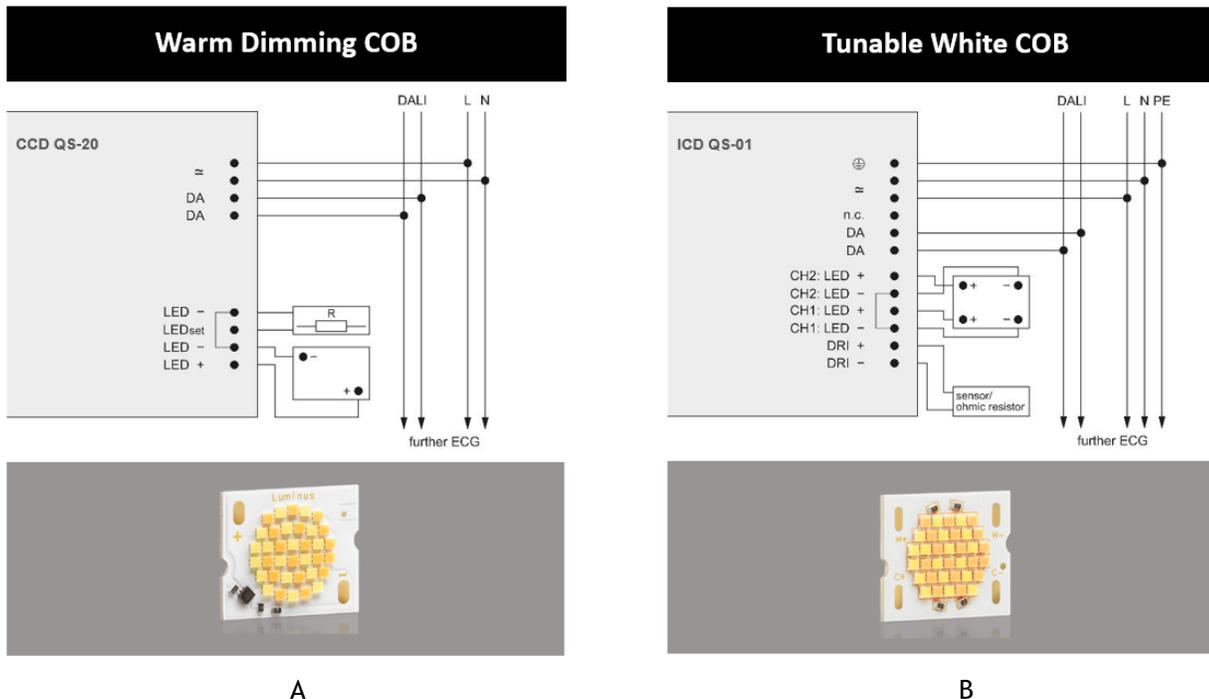
Figure 9: Wire Diagrams for Dynamic COBs
