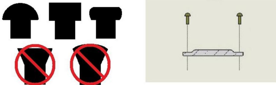
Figure 5: Screw Head Types and Screw Mounting
