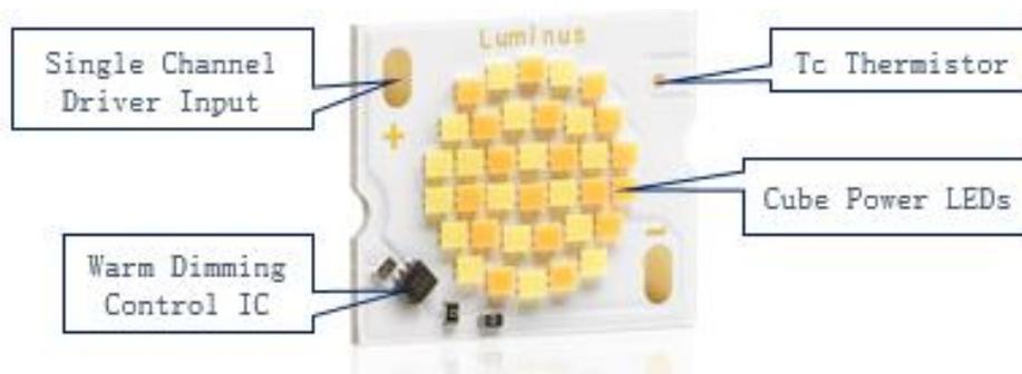
Figure 1: An Example of Warm Dimming COB
