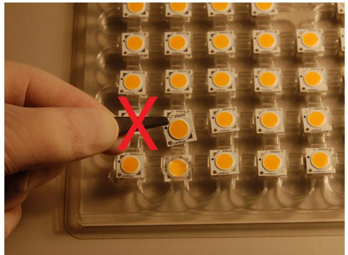
**Fig.5 Incorrect Handling**
