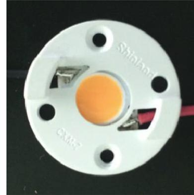
**Fig.11 Improper Centering of LES in Holder**
